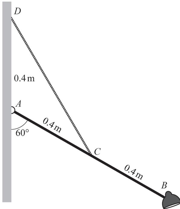
The diagram shows a wall-mounted light. It consists of a rod  $AB$  of mass  $0.25\text{ kg}$  and length  $0.8\text{ m}$  which is freely hinged to a vertical wall at  $A$ , and a lamp of mass  $0.5\text{ kg}$  fixed at  $B$ . The system is held in equilibrium by a chain  $CD$  whose end  $C$  is attached to the midpoint of  $AB$ . The end  $D$  is fixed to the wall a distance  $0.4\text{ m}$  vertically above  $A$ . The rod  $AB$  makes an angle of  $60^\circ$  with the downward vertical.
