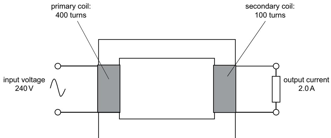
What are the output voltage across the secondary coil, the input current in the primary coil, and the output power of the transformer?
