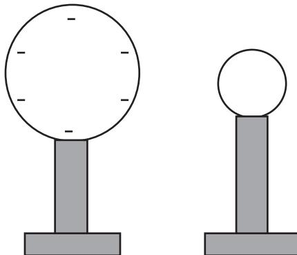
The smaller sphere is connected to the Earth by a conducting wire. Electrons flow from the smaller sphere to Earth because they are repelled by the larger sphere. The smaller sphere is then disconnected from the Earth.
