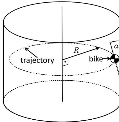
The bike and the rider are inclined at an angle  $\alpha$  to the wall. The angles  $\alpha$  that the bike can make with respect to the walls of the cage are limited by its handle bars to a certain minimum  $\alpha_{min} > 0$ . The tyres of the bike have a very high co-efficient of friction with the cage so that the tyres can only roll but not slip along the cage.
