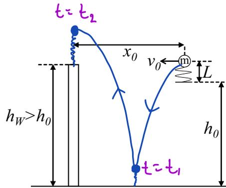
The above figure depicts a ball of mass  $m$  which is equipped on its lower side with a massless spring of uncompressed length  $L_0$  and spring constant  $k$ . The spring is initially compressed to a length  $L < L_0$ , as shown in the figure.
