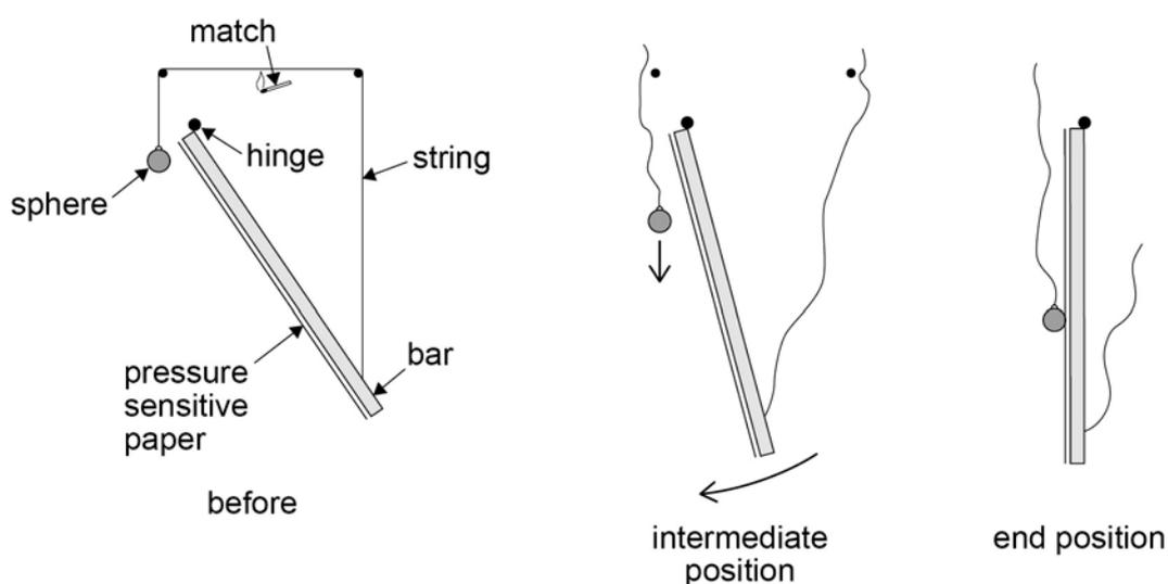
The student needs to measure the distance  $d$  fallen by the sphere in the time  $t$  taken for the bar to reach the vertical position.
