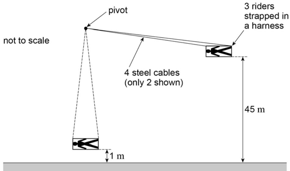
The harness in which three riders are strapped is supported by four steel cables. An advertisement for the ride states that the riders will be released from a height of 45 m above the ground and will then swing with a period of 14.0 s. It states that they will be 1.0 m above the ground at the lowest point and that they will travel at speeds of “up to 120 km per hour”.
