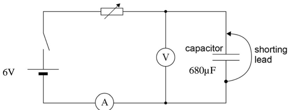
The variable resistor is then adjusted to give a suitable ammeter reading. The shorting lead is removed and the stop clock is started at the same instant.
