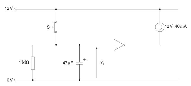
The CMOS inverting buffer (NOT gate) has the following parameters when connected to a 12 V power supply.
