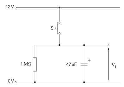
(a) Switch S is closed and then released at time t = 0. Determine the time taken for  $V_1$  to reach 6V. [2]
