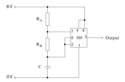
(a) The output signal has a mark:space ratio of 3:1. Sketch one cycle of the output signal. Label the  $\it mark$   $T_1$  and the  $\it space$   $T_2$ . [2]
