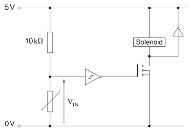
The solenoid is rated at 5 V, 3 A. Calculate the minimum value of  $g_{\rm M}$  required to allow the MOSFET to provide a load current of 3 A.
