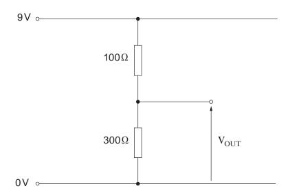
(a) Use Thevenin's theorem to produce an equivalent circuit.
