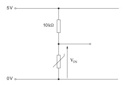
At 95°C the resistance of the thermistor is 2.3  $k\Omega.$  Calculate the value of  $V_{\rm IN}$  at this temperature. [1]
