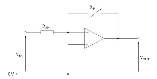
The input signal was set to amplitude 5 mV. The variable resistor was adjusted to give the output signal shown on the next page.
