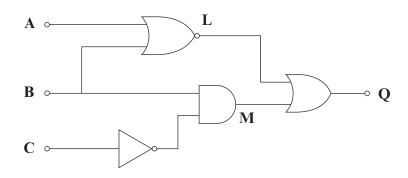
Write down Boolean expressions for the outputs L, M and Q in terms of inputs A, B and C.
