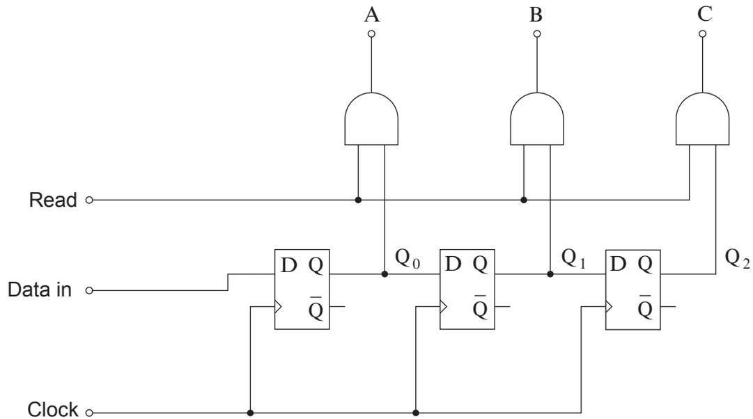
Complete the graphs opposite to show the outputs  $Q_0$ - $Q_2$ , and A-C in response to the given 'Clock', 'Data in' and 'Read' signals. [6]
