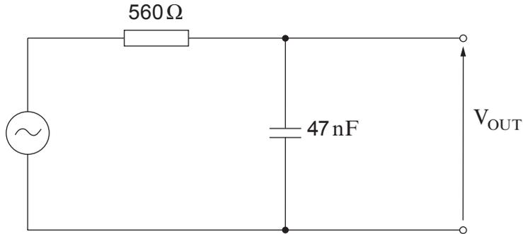
(a) What is the name of this type of passive RC filter? ..... [1]
