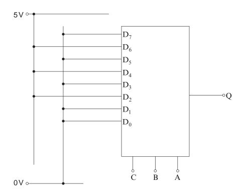
(i) Complete the truth table for the multiplexer shown in the diagram.
