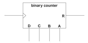
Complete the diagram to convert the counter into a BCD counter.
