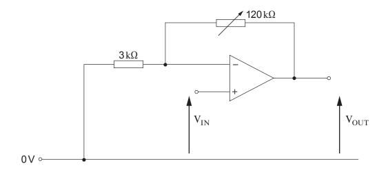
The op-amp is powered from a ±15 V supply and saturation occurs at ±14 V.
