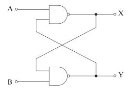
Complete the truth table to show the sequence of outputs at X and Y, for the given sequence of inputs. [3]
