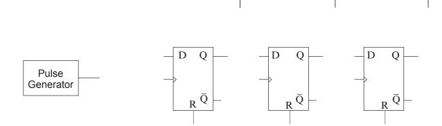
(b) The following circuit uses a 3-bit falling edge-triggered counter.
