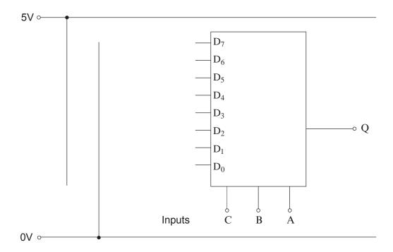
(c) The student tests the multiplexer sub-system using a LED. Add the necessary components to the diagram so that the LED is ON when Q is high (logic 1). [2]
