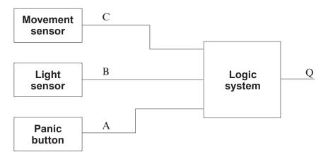
(i) Complete the truth table for the logic system such that  $\mathbf{Q} = logic 1$  when the floodlight is on. [1]
