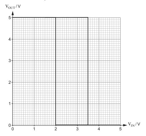
The Schmitt inverter is used to condition the signal produced by a sensing unit.
