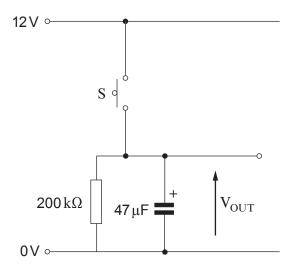
(i) Switch S is closed and then released at time t = 0. Calculate the value of  $V_{\rm OUT}$  at time t = 4 s. [2]
