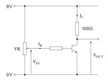
The output of the potentiometer VR is varied and readings of  $I_B,\,I_C,\,V_{IN}$  and  $V_{OUT}$  are taken.
