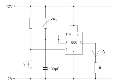
The timing sub-system consists of a  $100\,\mu\text{F}$  capacitor and a variable resistor  $VR_1$ . Calculate the resistance of  $VR_1$  so that a blue LED stays on for one minute after the switch S is momentarily pressed. [2]
