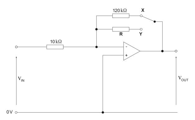
An input voltage of 0.8 V is applied to  $V_{\mbox{\scriptsize IN}}.$
