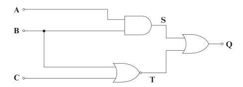
(a) Write down the Boolean expression for each of the outputs S, T and Q in terms of inputs A, B and C.
