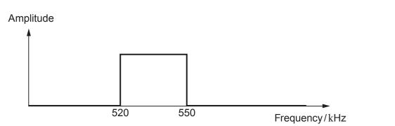
(a) A Frequency Modulated signal having the following frequency spectrum is connected to the input of the filter.
