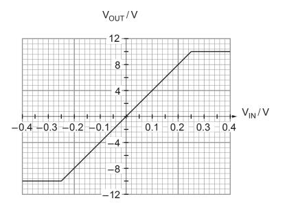
Design a voltage amplifier, based on a single op-amp that has this characteristic curve. Draw a fully labelled circuit diagram to show your design, showing clearly component values. [3]
