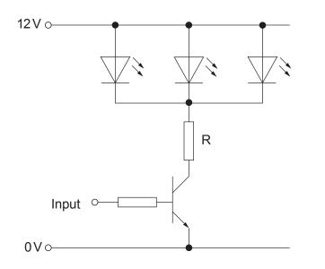
Each LED has a forward voltage drop of 2.5 V and a maximum forward current of 250 mA when lit. Calculate the value of resistor R needed to protect the LEDs when they are fully lit.
