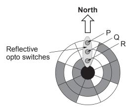
The outputs of P, Q and R are processed to light the appropriate LED on the display shown in the following diagram.
