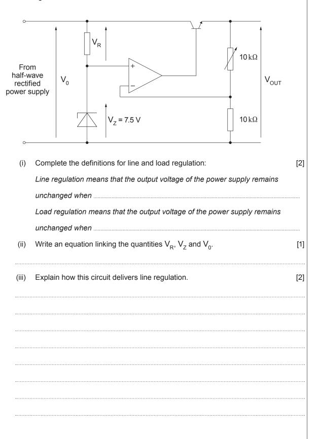
Examiner Calculate the maximum and minimum values of  $V_{\rm OUT}$  obtained by adjusting the variable resistor.  $$\rm I31$$ (iv) ..... .....
