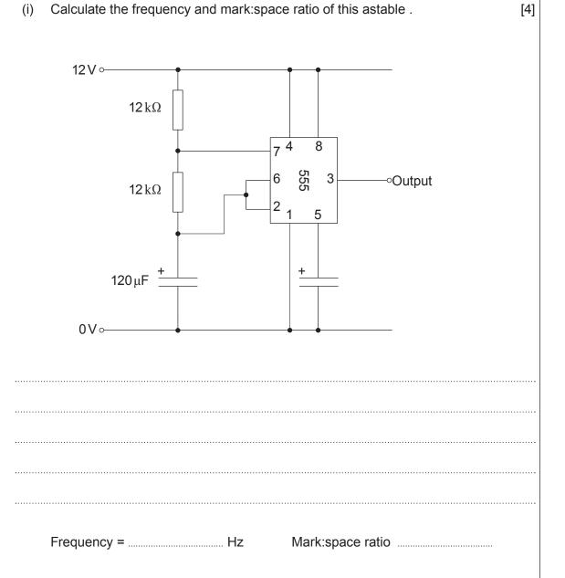
(ii) Using the axes provided, sketch a graph to show **two** cycles of the output signal produced by this astable, given that it pulses between 12 V and 0 V. [2]
