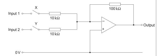
It is tested by applying a sine wave with an amplitude of  $0.5\,\mathrm{V}$  to input 1 and a steady DC voltage of +0.25 V to input 2. These are shown in the upper two graphs.
