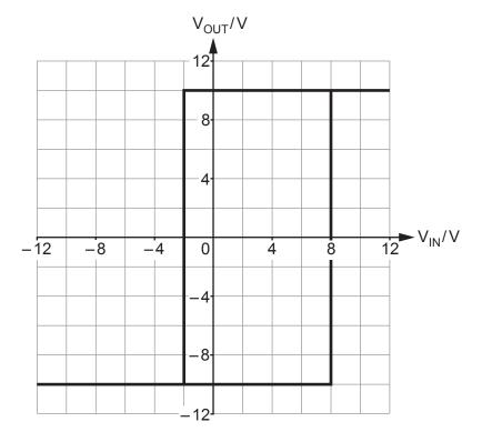
(i) For this Schmitt trigger, write down:
