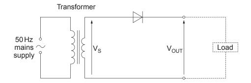
(a) On the axes provided below, draw a graph of the output voltage  $V_{OUT}$ . [2] The voltage,  $V_S$ , across the transformer secondary, is shown as a dashed line.
