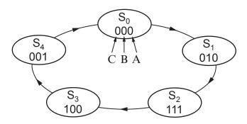
This control sequence is generated by a system of D-type flip-flops.
