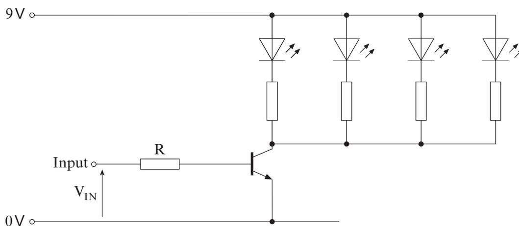
Complete the table with the word 'ON' or 'OFF' to show what happens to the LEDs for each value of  $V_{IN}$ .
