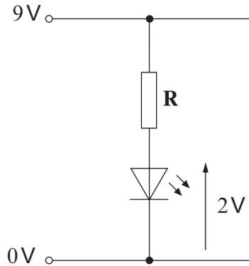
(a) What is the current through resistor **R** when the LED is lit? ..... mA [1]
