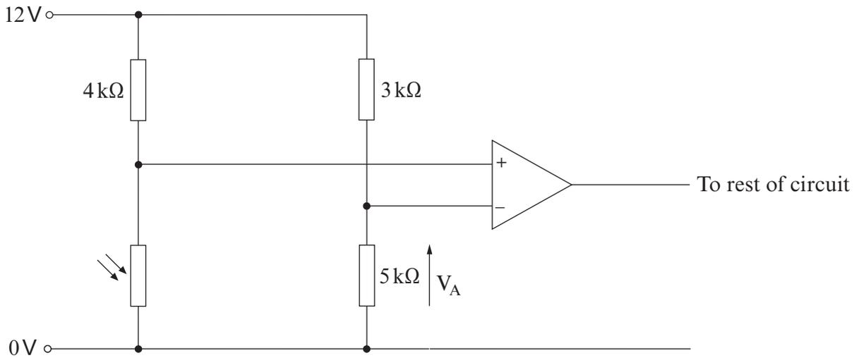
(a) (i) Which of the following is the correct formula to calculate the voltage  $V_A$ ?
