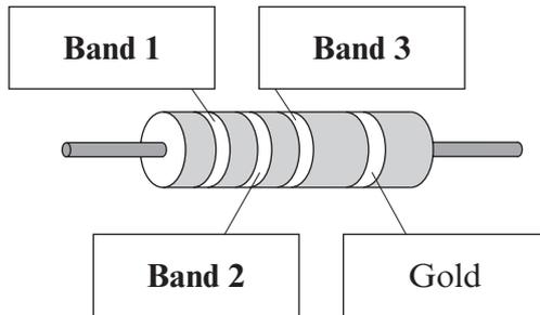
The resistor has a value of  $91 \Omega, \pm 5\%$ .
