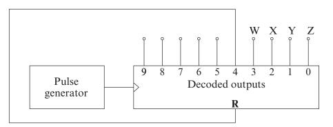
Reset input **R** is *active-high*, so the counter resets when **R** receives a logic 1 signal.
