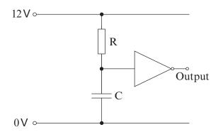
(a) Which combination gives the **shortest** time delay? (Tick  $(\checkmark)$  the correct answer.) [1]
