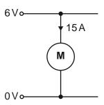
(a) Select the correct equation to calculate the power used in the motor in watts (W).(Tick (✓) the correct answer.)
