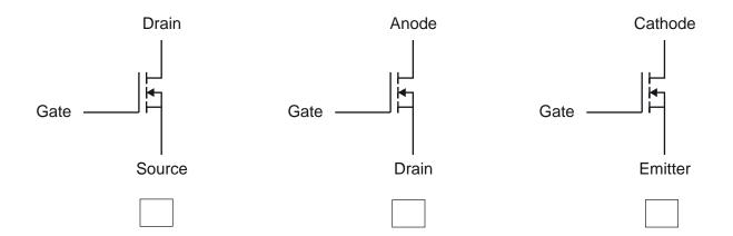
(c) The following diagram shows the circuit symbol for a thyristor.(Tick (✓) the correctly labelled symbol.) [1]
