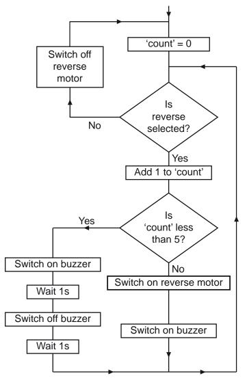
Reverse gear is selected. How many times does the buzzer pulse before the buggy moves?
