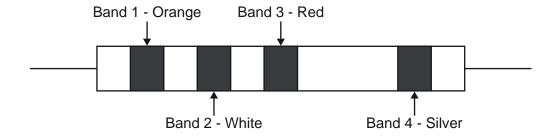
Circle the correct values for each band to show the value of this resistor in ohms.
