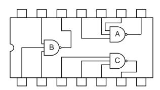
Tick  $(\mathcal{I})$  the box(es) for the input pin(s) for gate B. (b)
