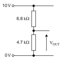
(i) Select the correct equation to calculate the voltage  $V_{
